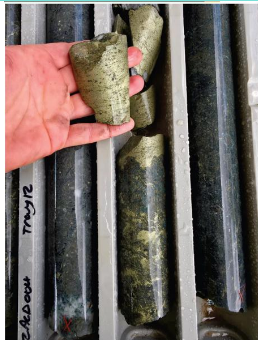
Figure 2: Chalcopyrite and pyrite sulphides in hole MZACD004
